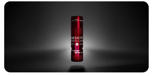
The SI-TL1 data logger is a small and compact multipurpose data logger for recording air pressure, height above sea level, temperature and 3-axis acceleration. With its size of only 53.5 x 15 mm and a weight of 19 grams, the SI-TL1 is very easy to attach or to be stored. The data records can be transferred to a computer via the SI-TL1 interface cable and then be analyzed with the free analyzing software.
